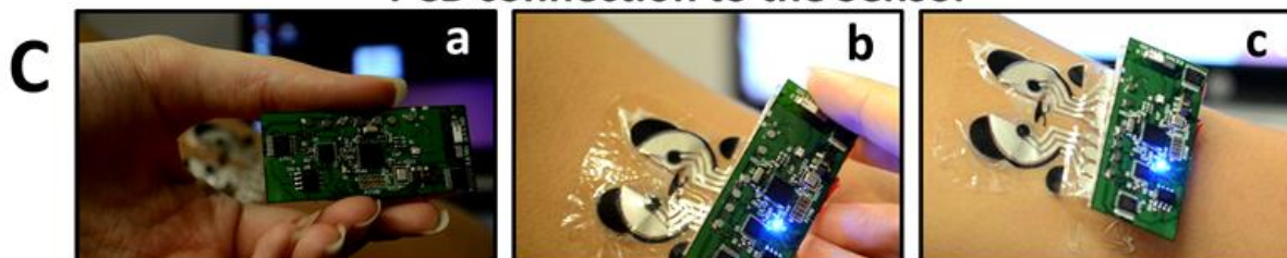
Figure S2: Tattoo transfer and PCB board integration for glucose and alcohol detection. A) Steps showing the process used to transfer the tattoo biosensor onto the skin. (a) Magnetic connections attached to the electrodes. Cathode and anode covered with PVA gel loaded with pilocarpine (left) and agarose gel (right), respectively. (b-c) Transferring the tattoo to the skin. (d-e) Releasing transferring paper using wet tissue. (f) Glucohol tattoo sensor on the skin. B) Electronics used to perform IP and chronoamperometry for glucose and alcohol detection. From left to right: Coin battery attached to the PCB, Magnets attached to the PCB's pad contact using a flexible plastic spacer to avoid the magnets to collapse. Front view of the PCB with magnets and battery on the back side. C) Magnetic attachment of the PCB board to the transferred tattoo.
