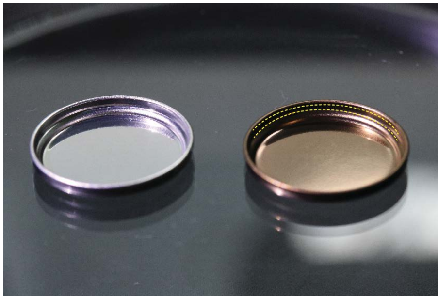
Supplementary Figure 13. Photograph of bare (left side) and TiN-coated (right side) stainless steel coin-type cells (bottom part). The edges of the custom-made TiN-coated stainless steel, where oxidation/corrosion of stainless steel takes place are indicated by yellow dash lines.
