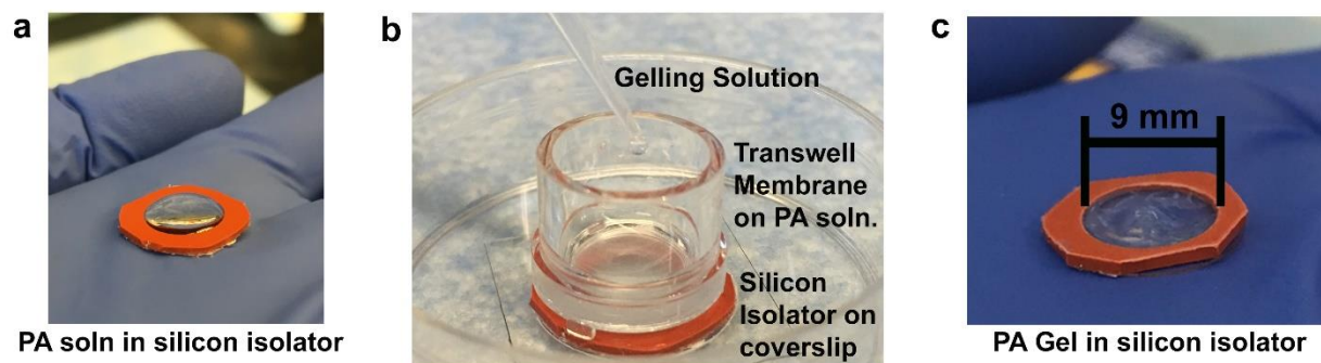
S15. PA Gel formation process. (a) PA gel solution is placed on glass coverslip within silicon isolator. (b) Transwell membrane is placed on top of PA solution and gelling solution is added through membrane. (c) PA gel molded to silicon isolator.
