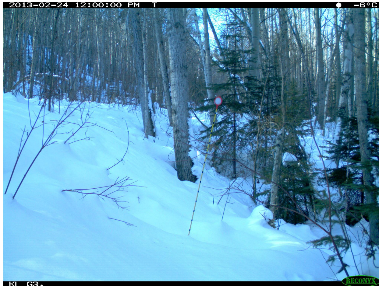
S1 Photo. Field set-up used to estimate snow depth with remote cameras. We estimated snow depth and snow accumulation by using remote cameras (Reconyx PC900, Reconyx Inc., Holmen, WI, USA) deployed across our study area. Cameras were programmed to take one picture every day at noon and were aimed at poles that were marked with black tape every 10 centimetres. We estimated snow accumulation by counting the number of black lines that were visible from one day to the next. Snow depth was estimated by adding initial snow depth (measured during deployment) to estimates of snow accumulation.
