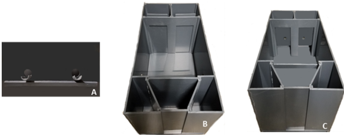
Supplementary Figure 4. Guessing task apparatus. A) back wall with goal holes; B) apparatus with guillotine doors closed; C) apparatus with guillotine doors open
