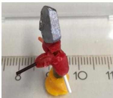
**Fig. S1. Optical image of big single crystals grown by self-flux method with congruent composition.** The flat cleaved surface on the left hand is the  $a$ - $b$  plane of the crystal.
