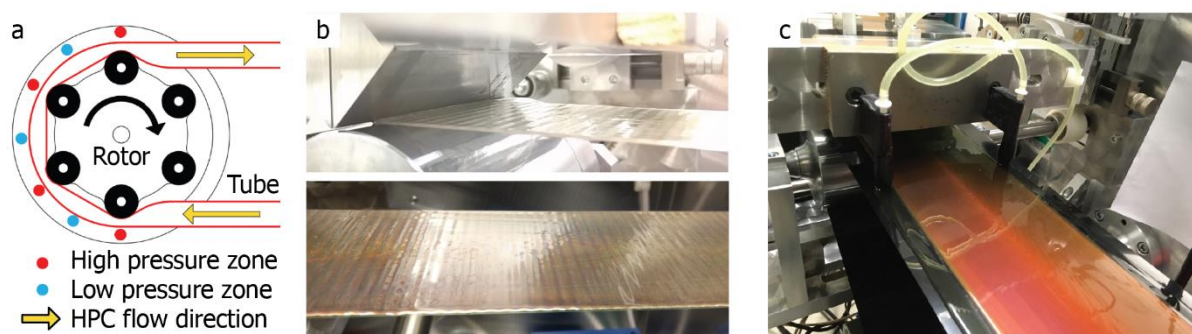
Supplementary Figure 4: a , Schematic of peristaltic pump: rotor periodically compresses tube to pump HPC inside. The intermittent pressure generated during fluid transport results in periodic fluctuations (“chatter” defects) in the HPC slot-die coating (b) . Pulsation is reduced by adding a pressure dampener along the pump line (depicted in Fig. 1a), ensuring homogenous coating (c) .
