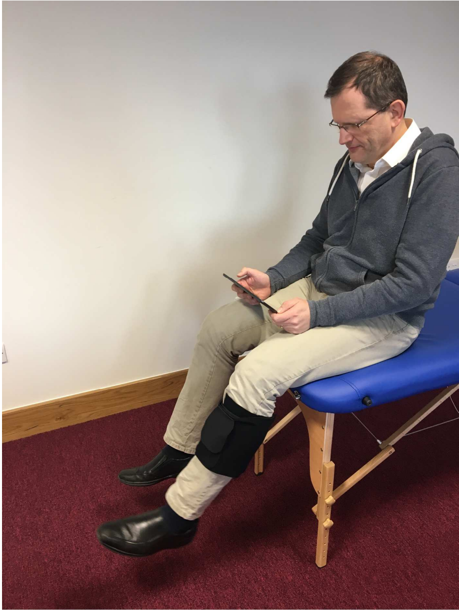
Figure 1: User setup of biofeedback system with single IMU placed on the shin and associated tablet application (written consent provided for use of image).
