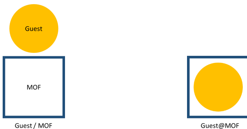
Figure S 5: Schematic illustration of the difference between a physical mixture of a MOF plus a guest material (left) and a Guest@MOF material (right) to illustrate the implication of the two scenarios on the BET surface area.
