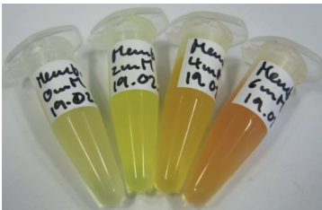
Fig. S4: Enhanced pigment production by L. chromiiresistens during chromate stress. Membrane fractions of cells grown with 0 mM, 2 mM, 4 mM and 6 mM K_2CrO_4 (left to right).
