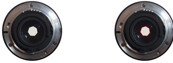
Figure B.1: Edge-detection of the exit pupil for an f/5.6 aperture. In the right image, in red: the edge-detected aperture shape.
