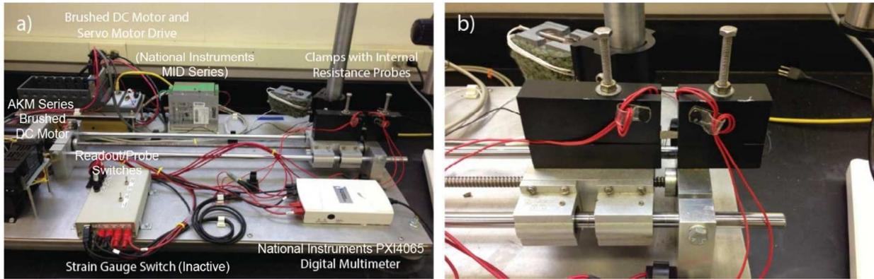
Figure S2: a) Custom-built 4 point-probe measurement system for tensile strain experiments. b) System applying strain while measuring electrical resistance using a 4 point-probe configuration.
