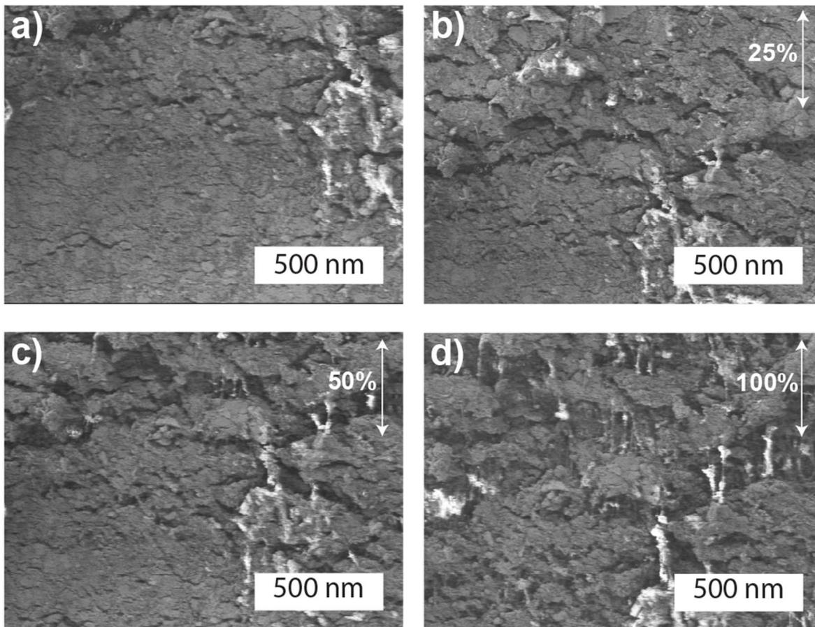
Figure S6: Low magnification SEM images of elastic conductors prepared from spinning solutions with 35% (wt/vol) Ag-PAA nanoparticle concentration under a) 0% strain, b) 25% strain, c) 50% strain, and d) 100% strain. The arrows indicate the direction of uniaxial tensile strain.
