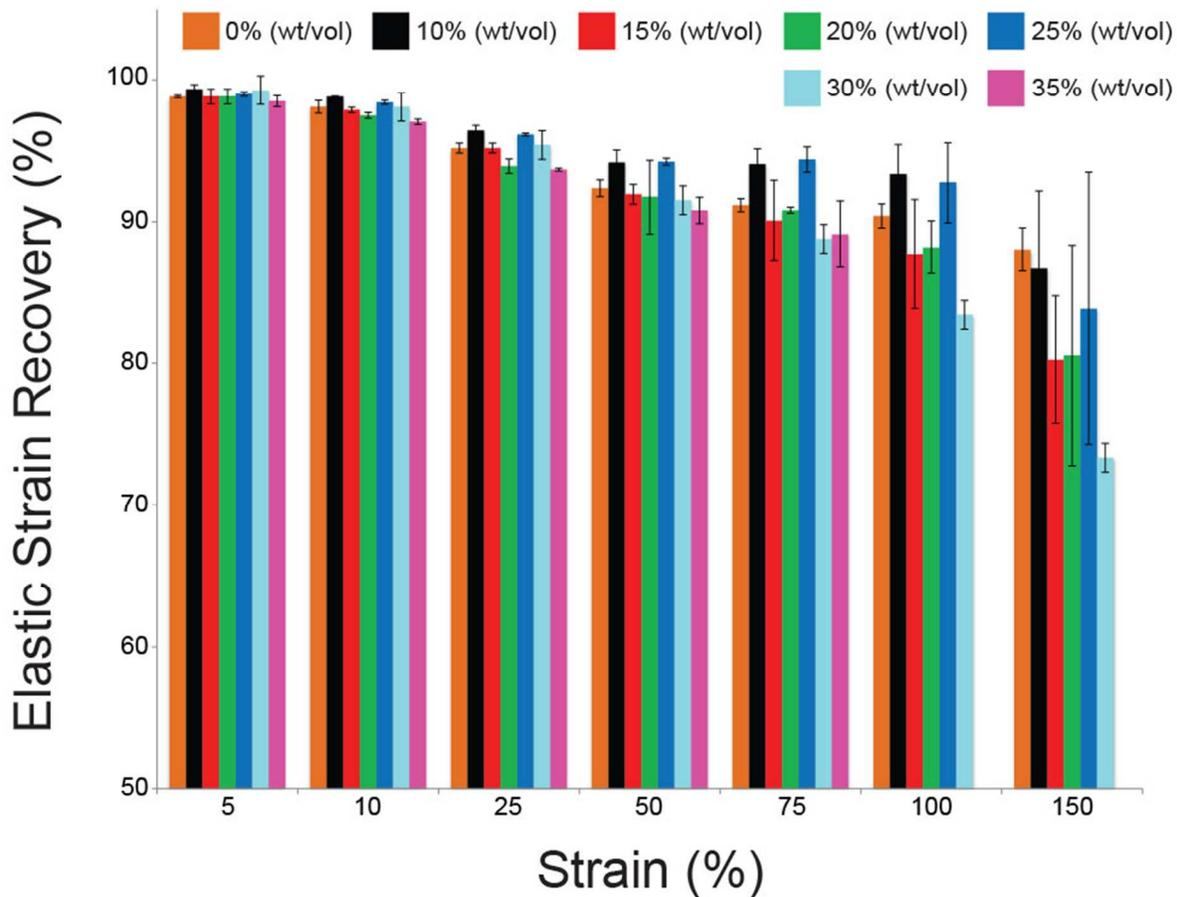
Figure S4: Elastic recovery of elastic conductors fabricated from block copolymer fiber mat (0%), and elastic conductors prepared from spinning solutions with different Ag-PAA nanoparticle concentrations after consecutive strain cycling to increasing maximum strain values. (number of samples is equal to 3 for all composites ( $n=3$ ), error bars represent standard deviation)
