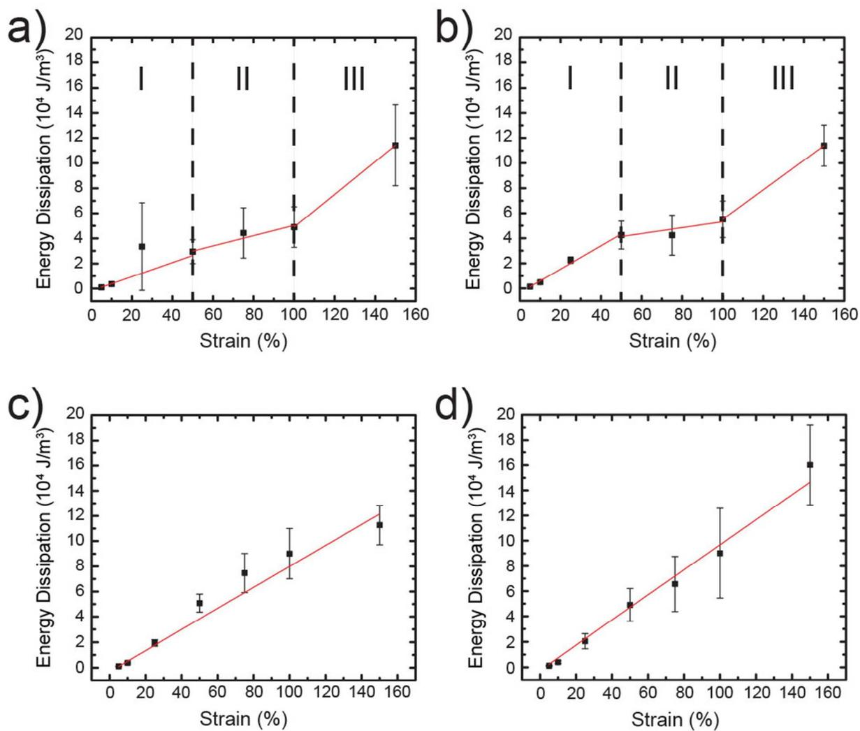
Figure S5: Average energy dissipation values and corresponding linear fits for elastic conductors prepared from spinning solutions with a) 15% (wt/vol), b) 20% (wt/vol), 25% (wt/vol), and 30% (wt/vol) Ag-PAA nanoparticle concentration. (number of samples ( $n=3$ ) is equal to 3 for all composites, error bars represent standard deviation)
