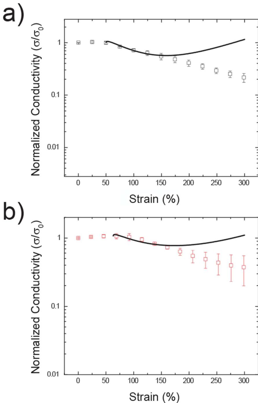
Figure S3: Experimental (data points) and theoretical (Equation 4) (black curves) normalized electrical conductivity ( $\sigma/\sigma_0$ ) dependence on strain for elastic conductors prepared using spinning solutions with a) 25% (wt/vol), and b) 30% (wt/vol) nanoparticle concentration under uniaxial tensile strain. (number of samples is equal to 3 for all composites ( $n=3$ ), error bars represent standard deviation)
