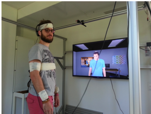
Figure 3. Picture showing the location of the 6 sensors (head, torso, both arms and forearms).
