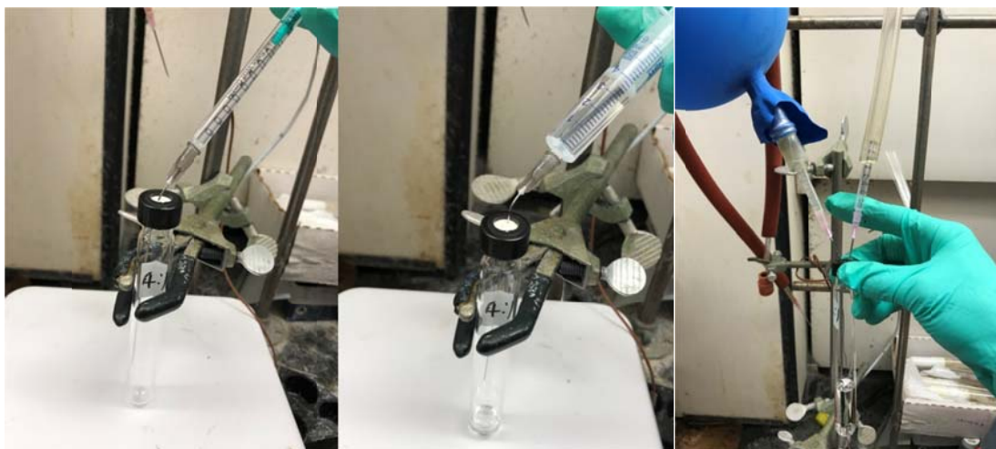
(Left) DMF (1 mL). (Center) Dioxane (4 mL). (Right) The mixed solvents were evacuated and backfilled with argon for twice.
