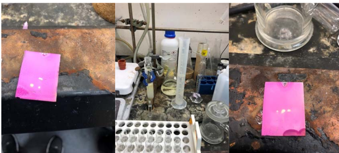
(Left) Crude TLC (right top spot is the product). (Center) Purification by flash column chromatography (silica gel). (Right) TLC after column.
