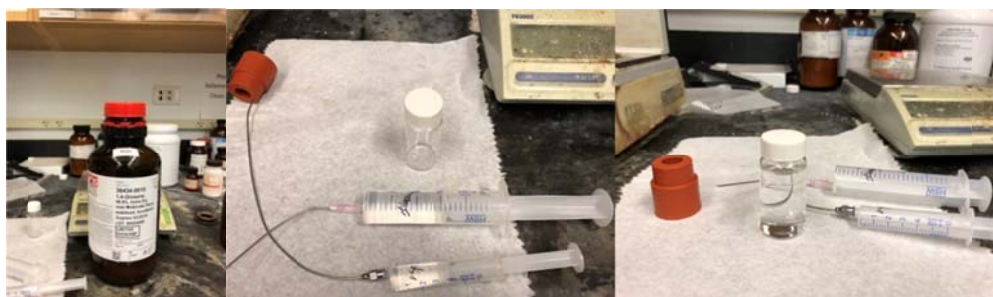
(Left) Dioxane (1 L sealed bottle, Acros). (Center) Prepare the solvent, DMF (4 mL), dioxane (16 mL). (Right) Premix the solvent in a 25 mL scintillation vial.
