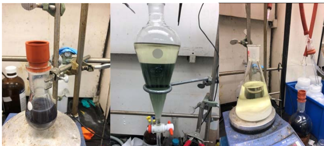
(Left) Quench the reaction by adding 10 mL \text{NH}_4\text{Cl} (aq) and 10 mL \text{Et}_2\text{O} . (Center) Transfer to a separation funnel. (Right) The organic phase was dried over anhydrous \text{Na}_2\text{SO}_4 .
