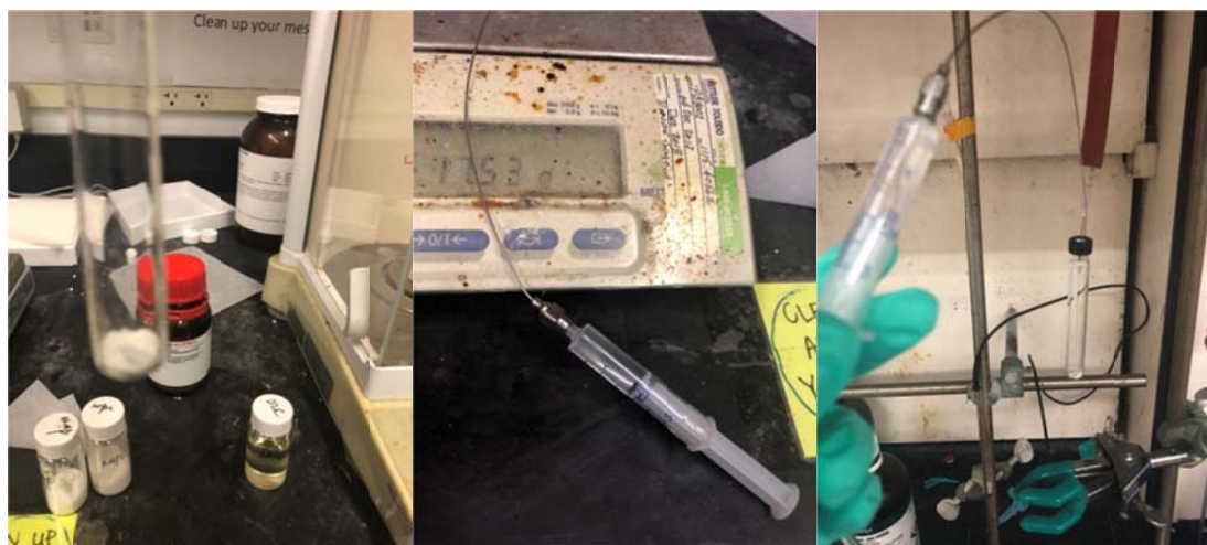
(Left) Add the acid and NHPI to a 15 mL culture tube. (Center) \text{CH}_2\text{Cl}_2 (2 mL). (Right) The tube was evacuated and backfilled with argon for three times and \text{CH}_2\text{Cl}_2 was added.
