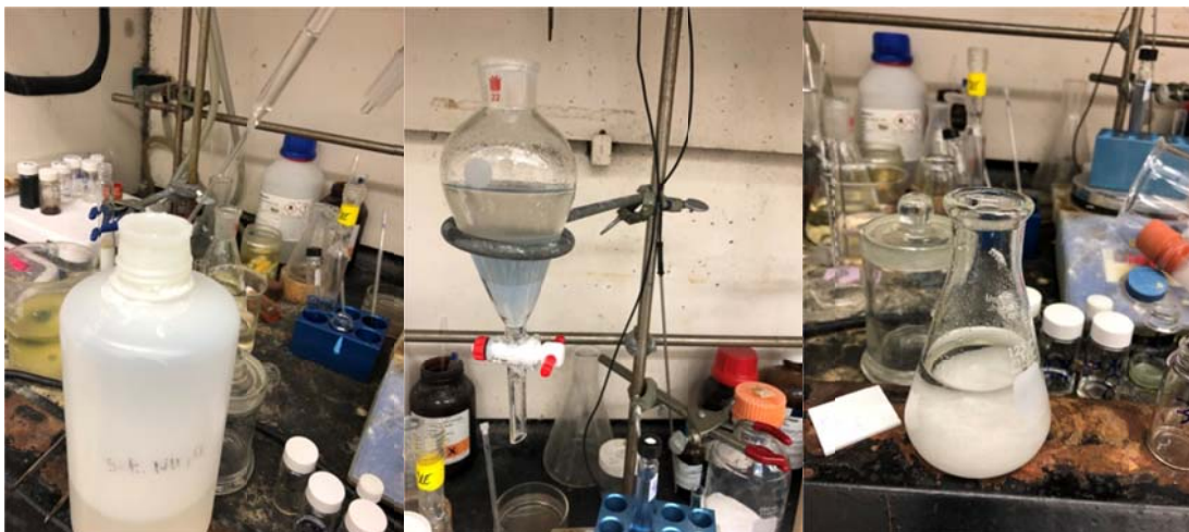
(Left) Quench the reaction with saturated \text{NH}_4\text{Cl} (aq) and EtOAc. (Center) Transfer the crude reaction mixture to a separation funnel. (Right) Organic phase was collected and dried over anhydrous \text{Na}_2\text{SO}_4 .
