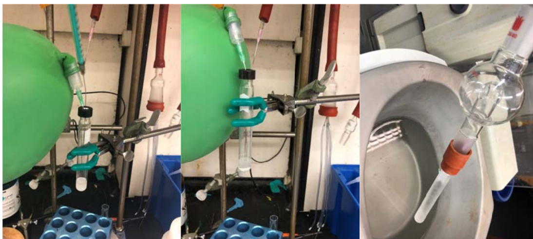
(Left) Add DIC (1.0 equiv). (Center) After stirring at RT for 2h. (Right) \text{CH}_2\text{Cl}_2 was removed by rotavapor.
