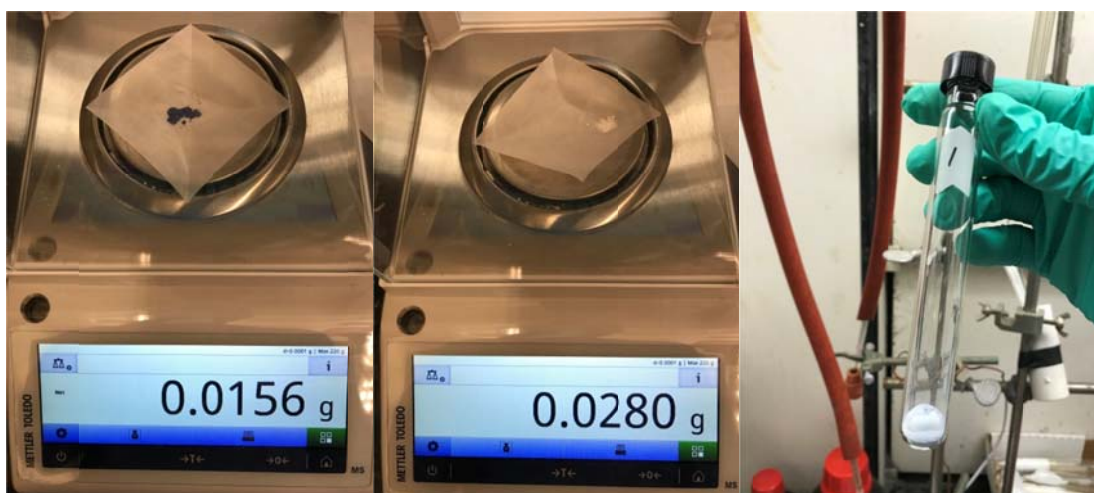
(Left) Cu(acac)_2 (30 mol%). (Center) MgCl_2 (1.5 equiv). (Right) Put all the five materials into a 15 mL culture tube equipped with a stir bar.
