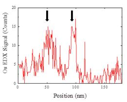
**Supplementary Figure S3**. (a) STEM HAADF image of a nuclear envelope showing the inner and outer membranes. The yellow line indicates the transect analyzed. (b) STEM-EDX Os content profile where two different Os peaks, corresponding to the inner and outer membrane, can be observed. N = nucleus, C = cytoplasm
