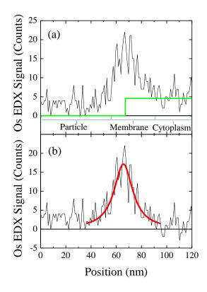
**Supplementary Figures S4**. (a) Os EDX signal (black) and its background signal (green). (b) Background-corrected Os EDX signal (black) with a fit to a Lorentzian function (red).
