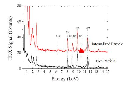
**Supplementary Figure S2**. EDX signal of the microparticle edge of a free microparticle (outside the cell) and an internalized one (inside an endolysosome). The Os peaks are only observed in the internalized microparticle. The peak highlighted in red was used to do the transient quantifications.
