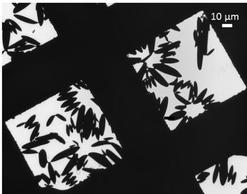
Supplementary Figure S6. PDLA microparticles without encapsulated AuNPs used for the background in the calibration curve (Figure S3).
