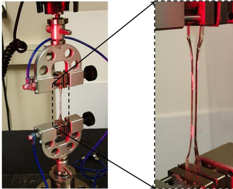
**Figure S3:** Material testing of dog-bone shaped 3DP-PDMS specimens using an Instron 5584H Load Frame equipped with a 50 N load cell to measure the Young's modulus and the elongation-at-break. (Inset) Magnified image of a specimen made of 3DP-PDMS with an E:S = 14 and TPO-L = 0.8% being subjected to tensile stress using the Instron 5584H Load frame.
