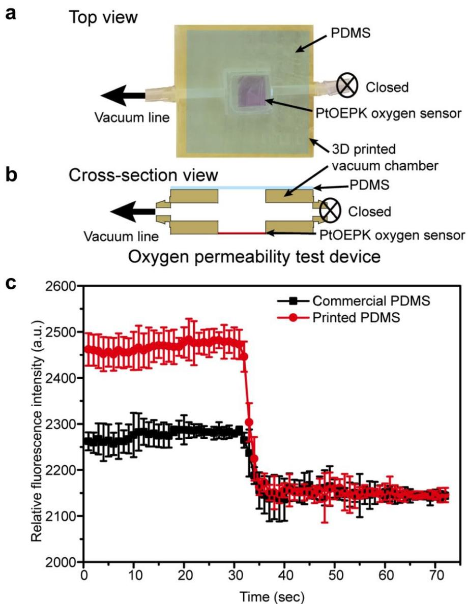
**Figure S7: Gas Permeability Measurements.** (a) Top view of the vacuum chamber device used for measuring the gas permeability of PDMS membranes. (b) Fluorescence intensity values measured every 1 sec as the chamber is allowed to equilibrate to atmosphere after being subjected to vacuum for 30 sec. Measurements were taken at 5 different positions on the sensor. The error bars denote standard deviation.
