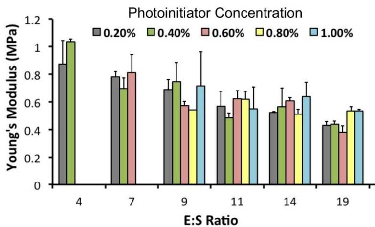
**Figure S4:** Young's modulus of 3DP-PDMS prepared with different ratios of end group and side-chain macromers, and different photo-initiator (TPO-L) concentrations. Error bars are standard deviations.
