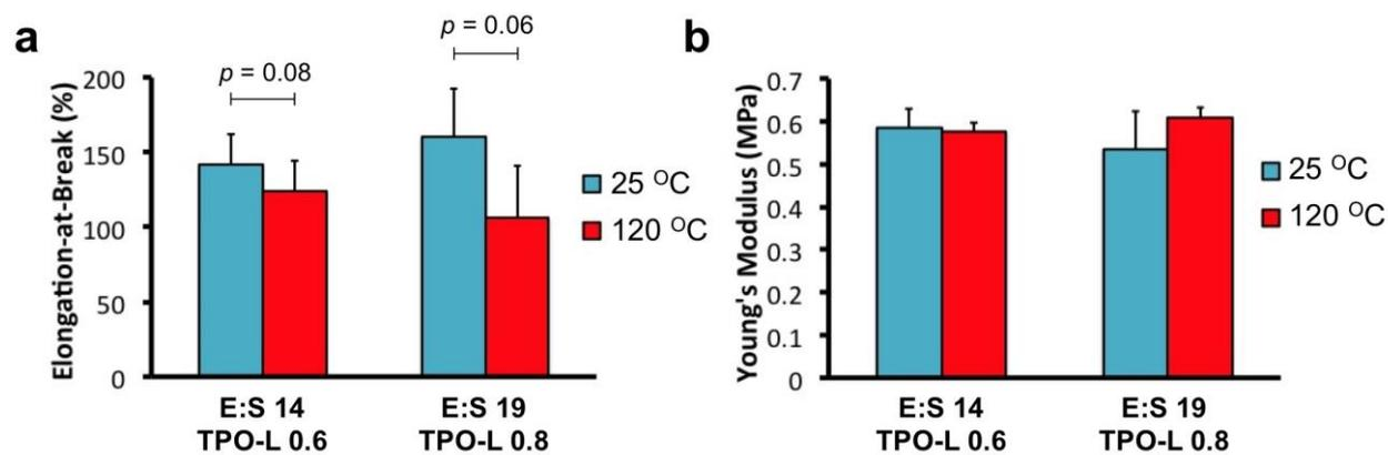
**Figure S5: Thermal Stability of 3DP-PDMS pieces:** (a) Elongation-at-break values and (b) Young's modulus of 3DP-PDMS dog-bone structures prepared with the two optimized Sylgard-184-like E:S blends and heated to 120 °C for 12 hrs. Error bars are SEM ( $n \geq 5$ ). Unpaired two-tailed Student's t-test did not show any significant difference between the elongation-at-break and Young's modulus means at 25 °C and 120 °C in either of the two E:S blends tested ( $p > 0.05$ ).
