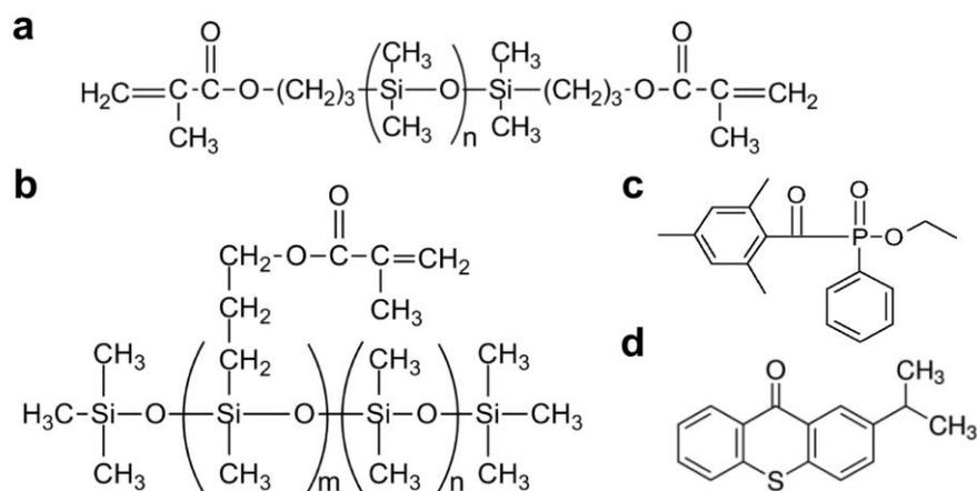
**Figure S1: Resin Components.** Chemical formulae of the resin components – (a) Macromer 1: end-terminated methacryloxypropyl poly(dimethyl siloxane), (b) Macromer 2: copolymer of methacryloxypropyl poly(dimethyl siloxane) and poly(dimethyl siloxane), (c) Photoinitiator: ethyl (2,4,6-trimethylbenzoyl) phenyl phosphinate (TPO-L) and (d) Photosensitizer: isopropyl thioxanthone (ITX).
