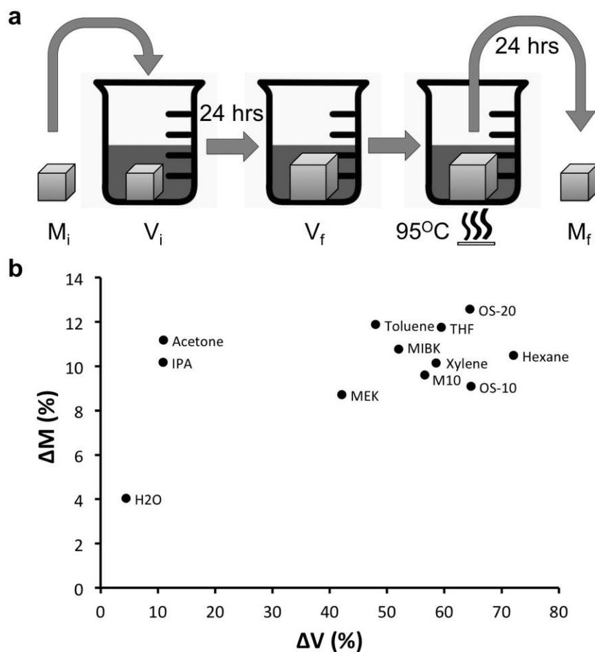
**Figure S6: Solubility of 3DP-PDMS-S in Organic Solvents.** (a) Schematic for measuring the swelling ratio and concomitant mass loss of 5 mm 3DP-PDMS-S cubes in different organic solvents. (b) Scatter plot of the change in mass (due to extraction) and the change in volume (due to swelling) of 5 mm 3DP-PDMS-S cubes in different organic solvents.
