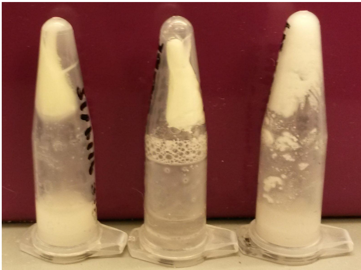
Figure S5. Examples of polymers that were phase separated at 37°C. Phase separation causing water excretion as well as opaque solids were observed with polymer solutions generated with a high amount of butyl methacrylate, high concentrations of polymer, and high PNIPAAm attachment to the functionalized HA.
