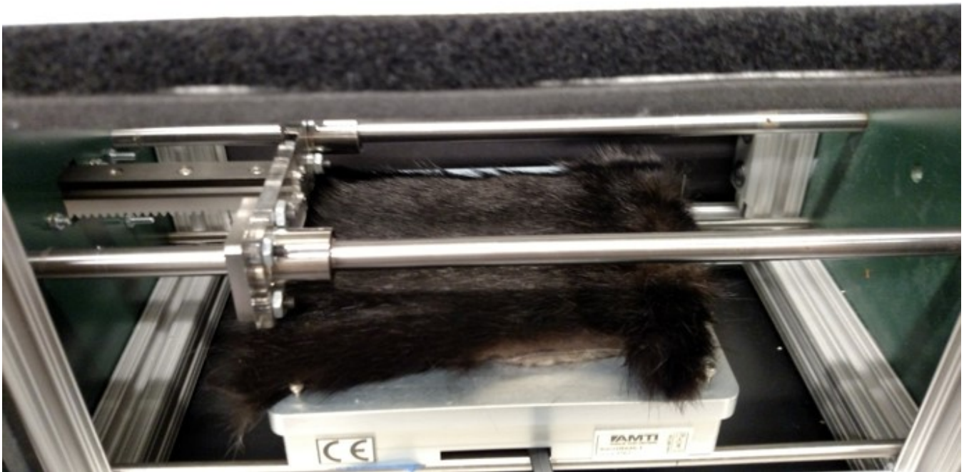
Fig. S2. Grooming machine. A cat tongue (top) is driven through a sample of cat fur (bottom) at a fixed velocity and fixed normal force of 0.1 N as measured by the AMTI HE6x6 force plate. The TIGR Brush and human hairbrush are also tested with the grooming machine.
