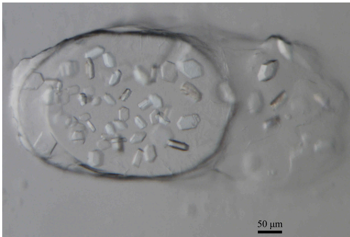
Figure S2. Image of a lipidic cubic phase (LCP) sandwich plate setup containing representative microcrystals of the hNK 1 R-PGS protein that were harvested to produce X-ray diffraction data.
