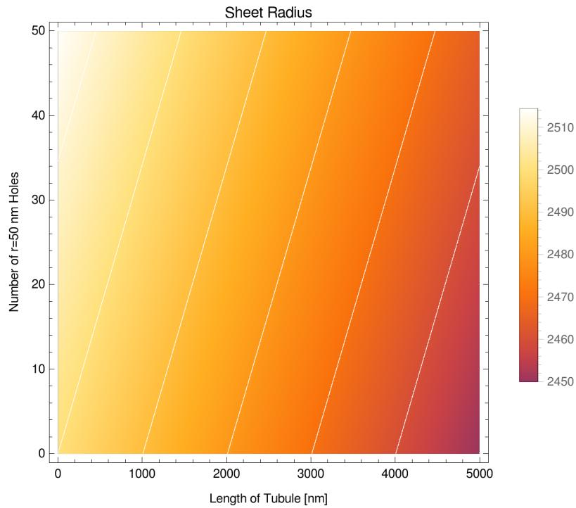
Initial sheet radius of  $2.5 \mu\text{m}$ , thickness of 50 nm
