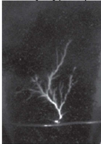
Figure S2: Laboratory based volcanic lighting (courtesy Betty Scheu and Donald Dingwell).
