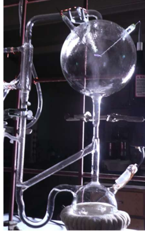
Figure S2: Laboratory based volcanic lighting (courtesy Betty Scheu and Donald Dingwell).
