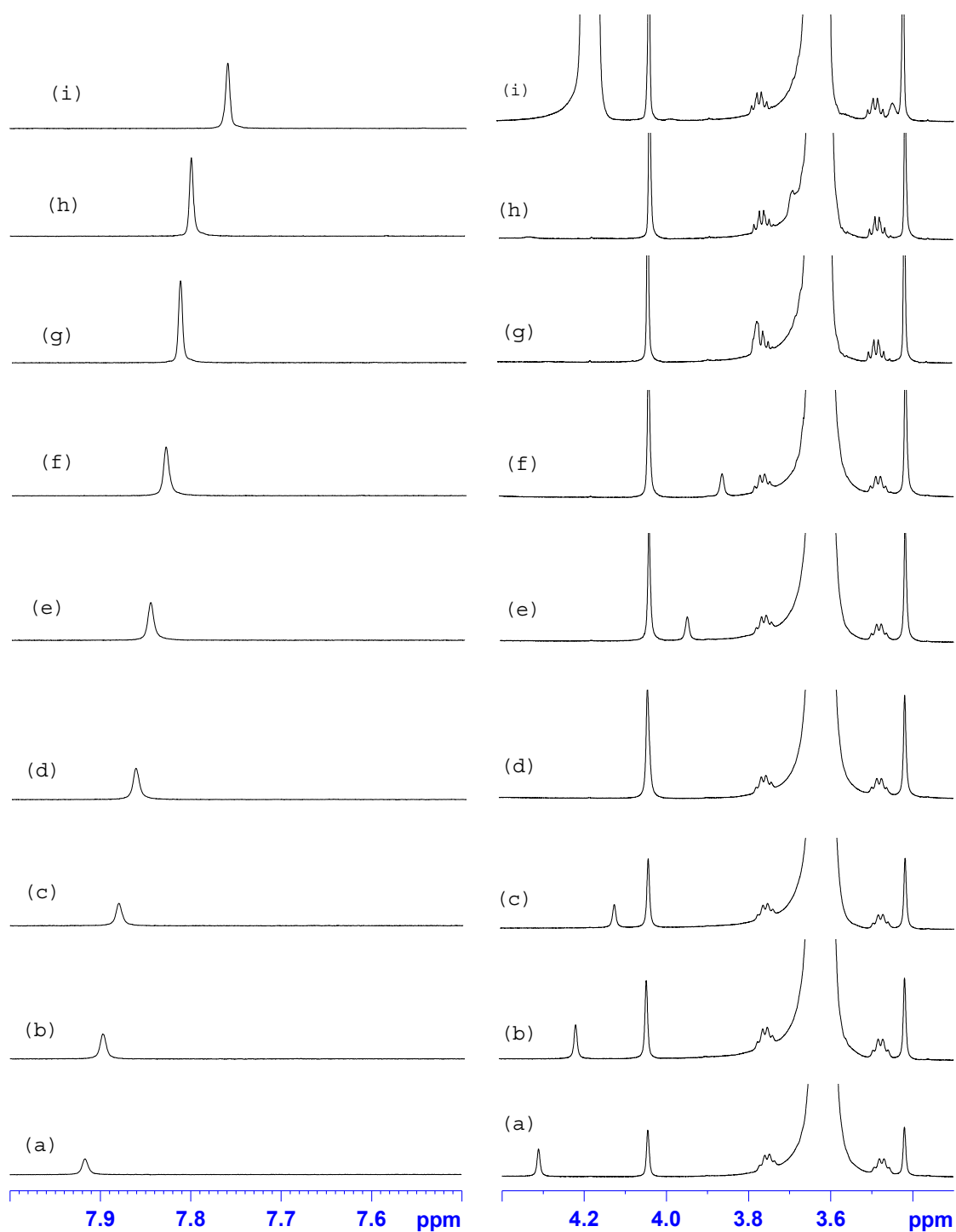
Figure S10. VT NMR spectra of 1-octanol gel of caffeine (a) 30 °C; (b) 35 °C; (c) 40 °C; (d) 45 °C; (e) 50 °C; (f) 55 °C; (g) 60 °C; (h) 65 °C; (i) 70 °C.
