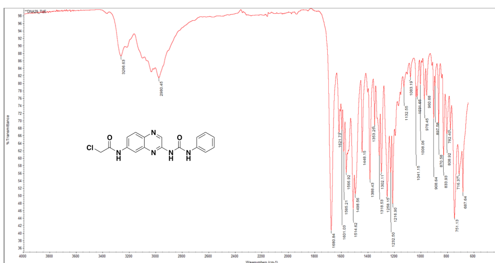
Figure S78. Infra red spectrum (ATR-FTIR) of compound 2-chloro- N -(3-(3-phenylureido)quinoxalin-6-yl)acetamide ( 7j ) (bands in cm -1 ).
