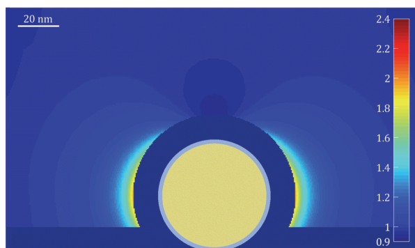
Figure S1: Numerical BEM calculations for both plasmonic sensors for a \varnothing 20 nm tethered sphere. (a) Scattering cross section in the proximal and the distal state of the tethered particle from a primary particle surface. Dashed lines represent optimum probe wavelengths. Spatial distributions of (b) plasmon shifts and (c) normalized intensity change at the probe wavelength induced by the tethered sphere (points in maps correspond to the geometrical center of the tethered sphere). The areas that the sphere cannot reach due to volume exclusion are visible as dark areas around the particles. Note that 2D projections are shown, whereas the calculations employ 3D distributions.
