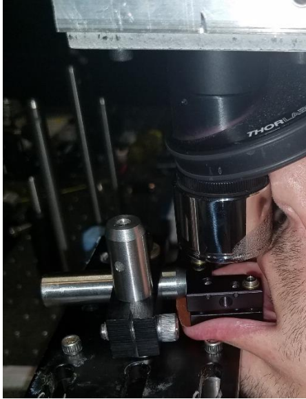
Figure S9 Procedure of in vivo human imaging of labial mucosa. Lip was clamped down and sandpaper is used on clamp to prevent slippage. A hand-driven stage allows for fine adjustment of lip location.
