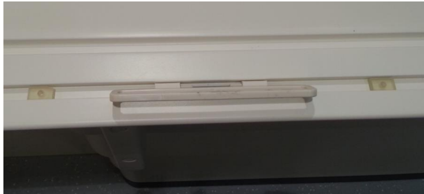
Pictured above: One side of the MRI table with the soft-strap holder in-between the two slide-in table inserts.
