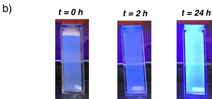
**Figure S7.** Biotinylated Initiator **7** Initiates Fluorogenic ATRP Polymerization. Emission spectra (a) and photos (b) of Anthracene:PEG Co-Polymerization at indicated times following excitation at 371 nm (a) or by hand-held UV lamp (b).
