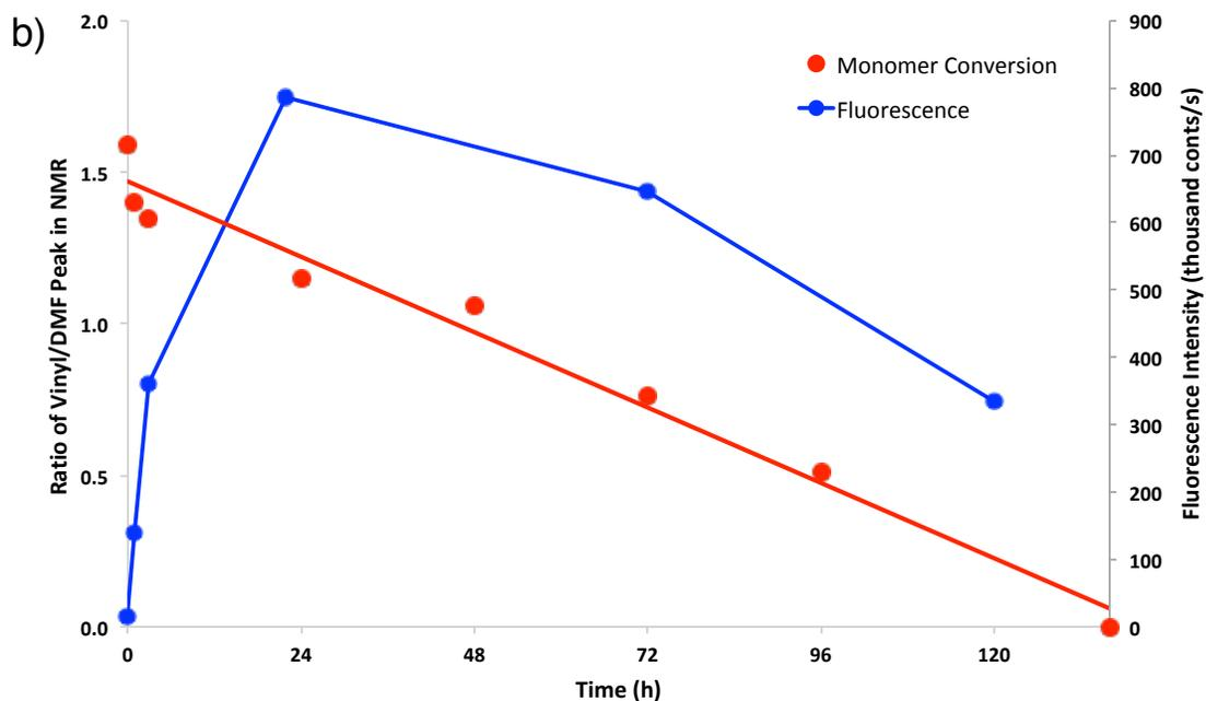
**Figure S1.** Monomer Conversion to Polymer is Observable with Proton NMR Analysis and Fluorescence Tracks with Early Monomer Conversion. a)  $^1\text{H}$  NMR spectrum of fluorogenic ATRP polymerization reaction at  $t=0$ . b) Graph of vinyl peak/DMF peak ratio of areas measured by  $^1\text{H}$  NMR and anthracene fluorescence at 426 nm following 371 nm excitation at indicated time points.
