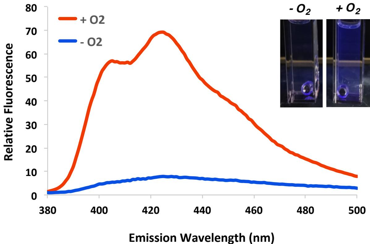
**Figure S6.** Trace Oxygen Initiates ATRP Polymerization in the Absence of Initiator. Plot of fluorescence emission and pictures of reactions run with anthracene:PEG co-polymerization at  $t = 24$  h with no initiator **4** in the presence (no degassing, + O<sub>2</sub>) and absence (with 1 h degassing under N<sub>2</sub>, - O<sub>2</sub>) of oxygen following 371 nm excitation.
