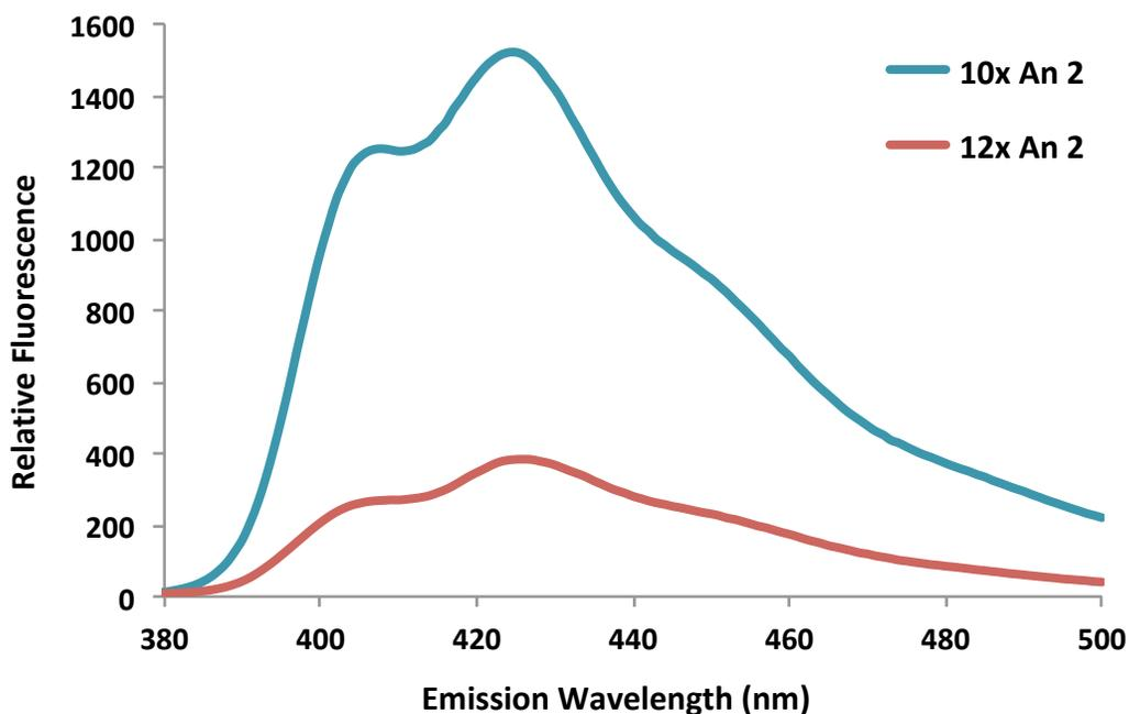
**Figure S3.** 10-Fold Anthracene Incorporation Over Initial Conditions are Optimal for Fluorescence Output. Emission spectra at  $t = 22$  h of various fold increases in anthracene monomer (**An 2**) incorporation in ATRP co-polymerization following 337 nm excitation.
