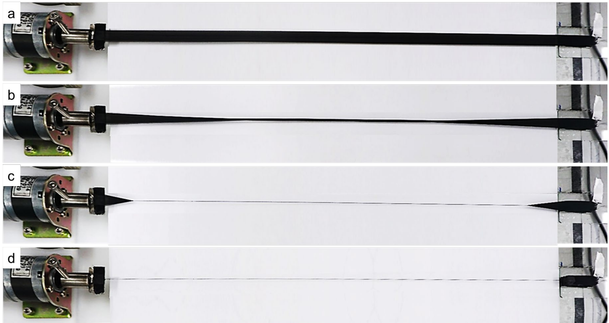
Supplementary Figure 1. Photographs of CNT sheets wrapping process on the stretched ( \epsilon_{fab} = 400\% ) spandex core fibre
