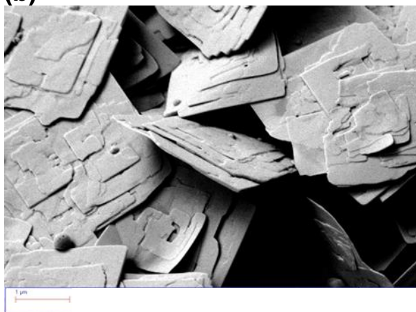
Figure S15. Additional SEM images of (a) dilute and (b) concentrated drop-cast 2D SnS square nanosheets.
