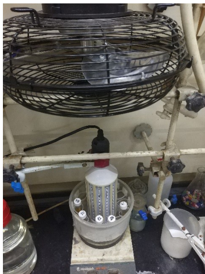
Figure S1 Photograph of the Photocatalytic reactor used for reactions conducted under blue LED irradiation.
