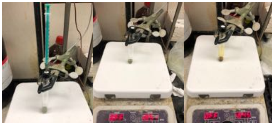
(Left) After addition of NMP. (Center) Crude mixture as reaction started. (Right) Crude mixture as reaction ended (6 h).
