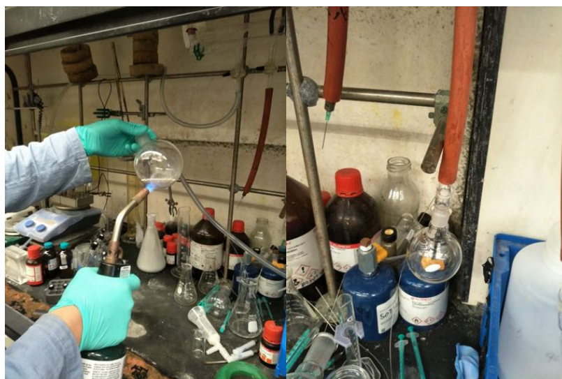
(Left) Activation of molecular sieves by flame-drying. (Right) The round-bottomed flask dried under vacuum.
