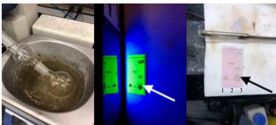
(Left) Organic layer was concentrated. (Center) TLC (hexanes 4:1 EtOAc, UV). Left lane: redox-active ester. Center lane: sulfinimine. Right lane: crude mixture. The
