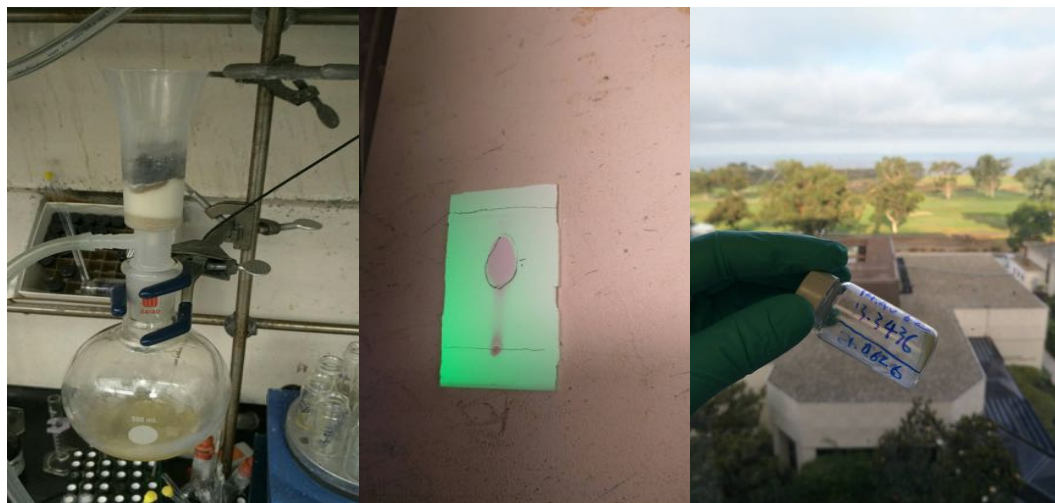
(Left) Filtration through a short pad of Celite ® . (Center) TLC ( \text{CH}_2\text{Cl}_2 , UV) of the crude mixture (stirring at rt overnight), (Right) Product (white solid) after short column.
