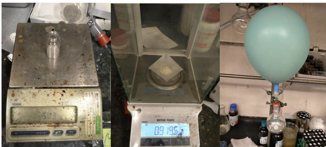
(Left) Molecular sieves. (Center) Sulfinamide. (Right) After addition of molecular sieves and sulfinamide, flask was placed under Ar atmosphere.
