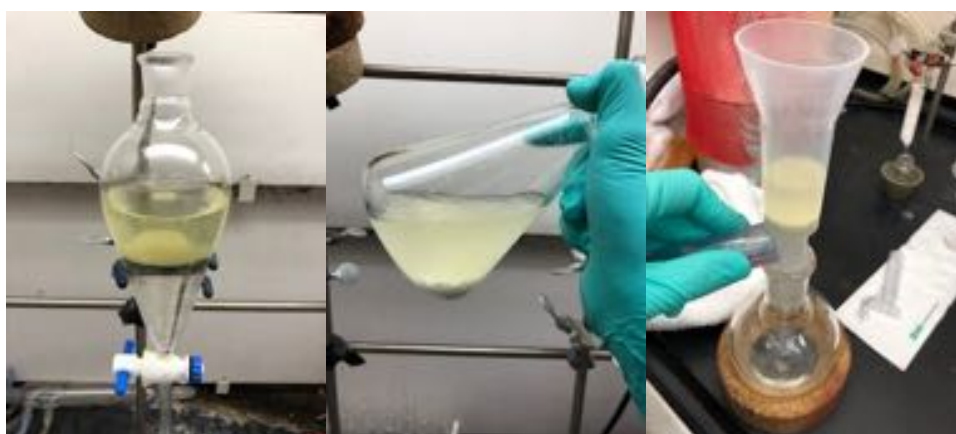
(Left) Crude mixture was diluted with EtOAc and extracted with water and brine. (Center) Organic layer was dried over \text{MgSO}_4 . (Right) Organic layer was filtered.
