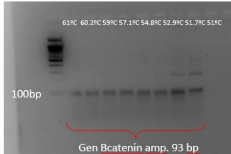
Figure 3. Electrophoresis 2% agarose, 100V, 70 min. \beta -catenin gene presented unspecific bands when we working with annealing temperatures of 51 – 52°C.
