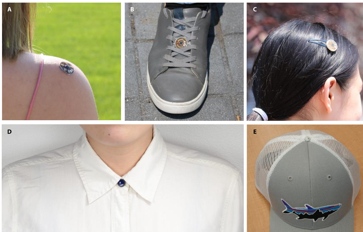
Fig. S2. Millimeter-scale, battery-free wireless sensors of UVA/UVB radiation. (A) Photographic images of mm-NFC UVA/UVB dosimeter as a skin patch mounted on shoulder, (B) mm-NFC UVA/UVB dosimeter as a shoe clip, (C) mm-NFC UVA/UVB dosimeter as a hair clip, (D) mm-NFC UVA dosimeter as a button, and (E) mm-NFC UVA dosimeter integrated into a hat.
