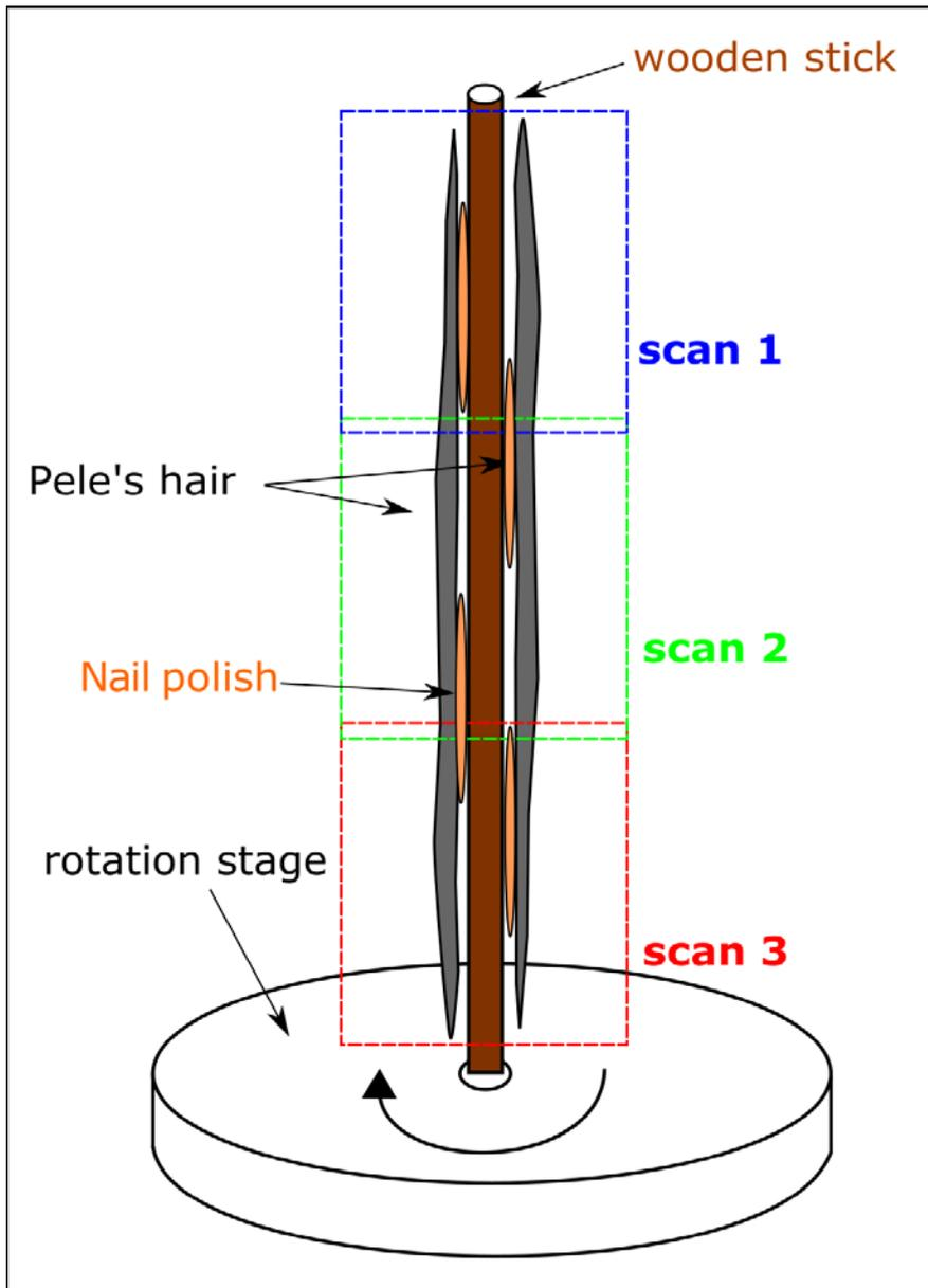
**Supplementary Figure S7:** Schematic example of the multiple scans analysis. Typically, 4 to 6 Pele's hairs were glued with nail polish to a wooden stick and mounted with their elongation axis parallel to the rotational axis of the rotation stage. Multiple scans were performed with an overlap of  $\sim 0.3$  mm between two consecutive scans.
