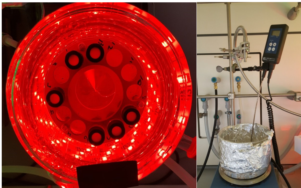
Figure S1. In-house light set up consisting in a jacketed beaker with LEDs winded around (left) and white light set-up consisting on a water bath light beam coming from the top via an optic fiber (right). Photograph taken by S.J.-P. Willot.
