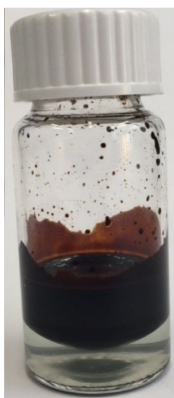
Figure S1 Visual appearance of the liquid products after the catalytic hydrotreatment reaction.
