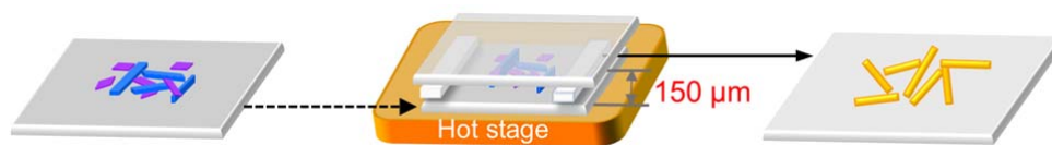
Figure R4. MAS apparatus for growth of 1D FTCs.
