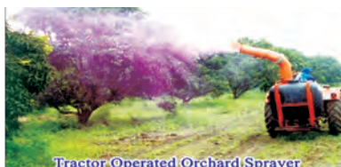
Aero Blast Sprayer for tall crops, and trees
