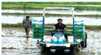
Self Propelled Paddy Trans-planter
