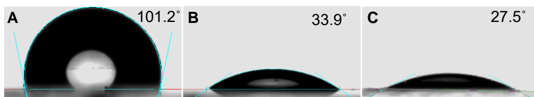
Figure S6. Water contact angles of (A) PBDTBT-C6C10, (B) PBDTBT-4EO, and (C) PBDTBT-7EO films, related to Figure 1.
