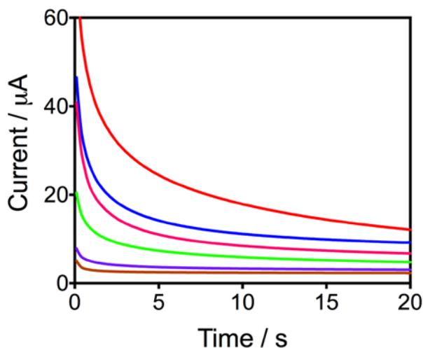
**Fig. S2** Chronoamperometric curves for various concentrations of PSA antigen (ascending along y-axis): 0, 0.001, 0.01, 0.1, 1 and 10 ng/mL in human serum samples containing 4.5 mM hydroquinone and 0.1 mM  $H_2O_2$  solution in CASPE-MFD at -2.0 mV step potential (vs. a silver pseudo-reference electrode).
