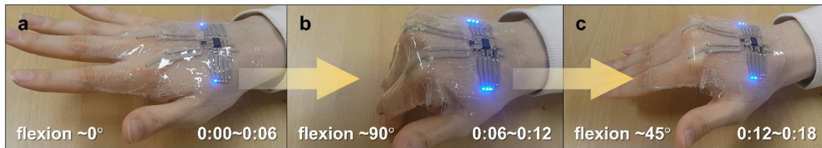
Figure S11. Calibration process of a MP joints flexions monitoring device. Calibration begins when the external power is applied. Right after that, the LED display block blinks for (a) one, (b) three, and (c) two LEDs for 6 seconds each, indicating that calibration is in progress. We asked the subject to bend the MP joints at 0, 90, and 45° at each step (a-c).
