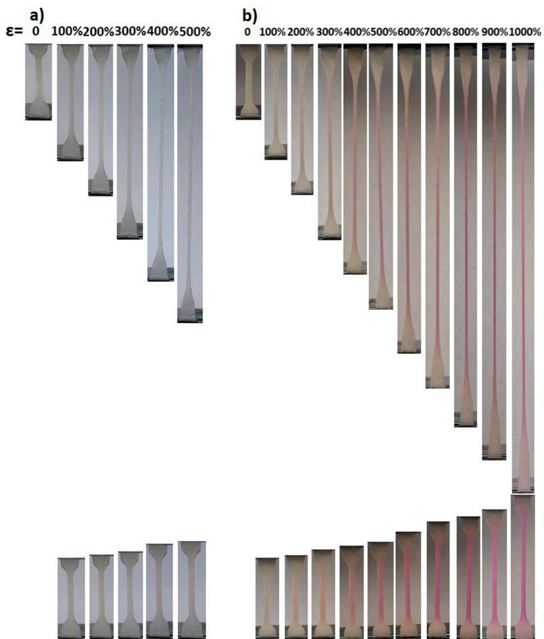
Figure S9. Optical images of a) poly(AAm-co-MA 0.5 -co-C12 0.5 /Rh) and b) poly(AAm-co-MA-co-C18/Rh) with a solid content of 70 wt% at both stretched state and the corresponding relaxed state.
