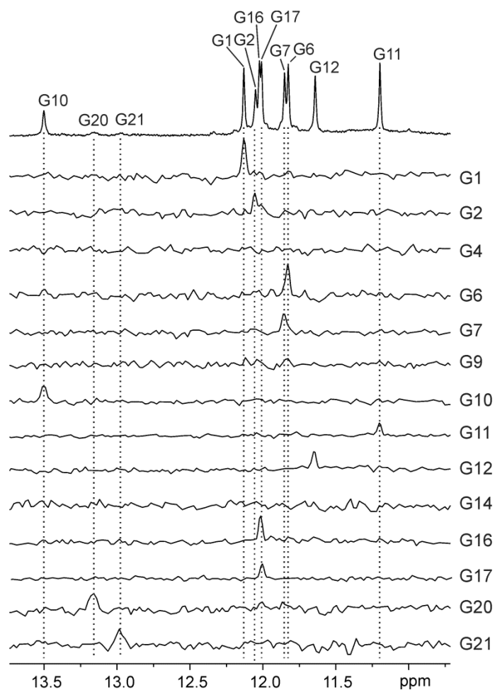
Figure S10. Imino region of ^1\text{H} and 1\text{D } ^{15}\text{N} -edited HSQC NMR spectra of kit* at 37^\circ\text{C} . The HSQC spectra were acquired on partially (10%) residue-specifically ^{15}\text{N} - and ^{13}\text{C} -labelled oligonucleotides. Assignment of H1 proton resonances is indicated on the right of each 1D HSQC spectrum. NMR spectra were recorded at 0.5 mM kit* concentration per strand, 100 mM KCl, pH 7.4 on a 600 MHz spectrometer.
