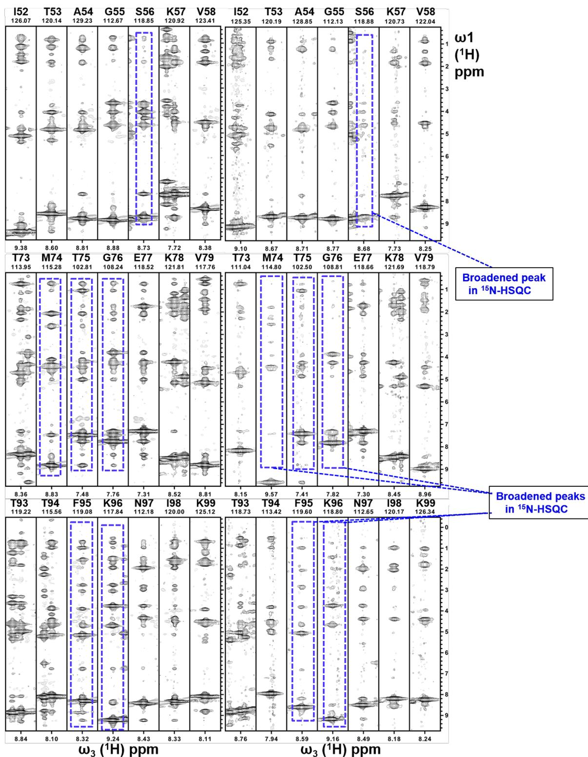
**Supplementary Figure 12.** 2D [ $^1\text{H}$ , $^1\text{H}$ ]-NOESY strips from 3D  $^{15}\text{N}$ -resolved-[ $^1\text{H}$ ,  $^1\text{H}$ ]-NOESY from [ $^{13}\text{C}$ ,  $^{15}\text{N}$ ]-labelled FABP1 in the absence (left) and presence (right) of GW7647. Several amide proton resonances are broadened in the presence of GW7647.
