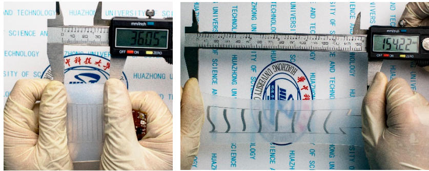
Figure S1. The photographs of the device before and after stretching, which demonstrate that the ultimate tensile capacity of the device can reach 300%.
