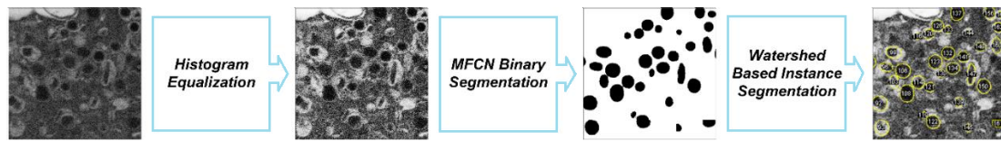
Figure S1. Flow diagram of whole image processing procedure. Whole image processing can be divided into three parts: histogram equalization, MFCN binary segmentation, and watershed-based instance segmentation.
