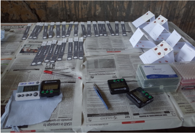
Photo ESI-5 Origami tests for testing in the school with and FTA blood-spots on cards for retrospective analysis using PCR at the University of Glasgow
