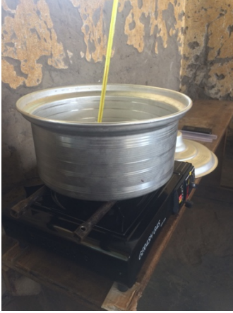
Photo ESI-7 Frugal testing using a local cooking stove to run LAMP amplification using manual control of temperature.
