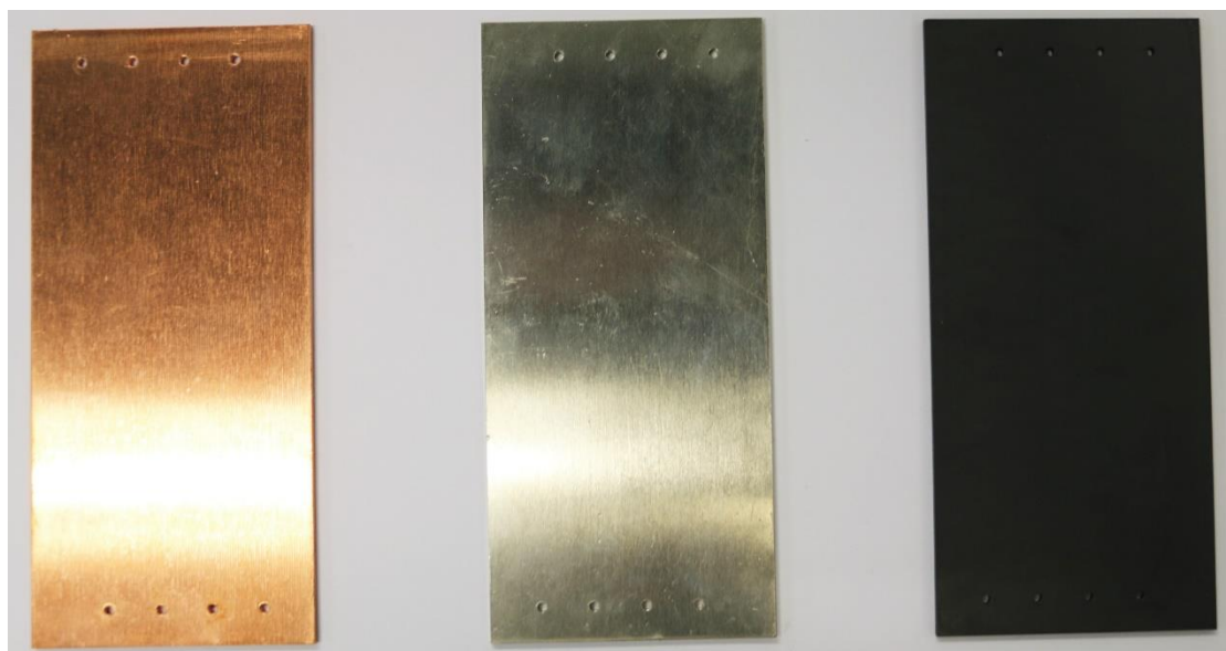
Figure S5. Copper (left), stainless steel (middle) and graphite (right) electrode plate.
