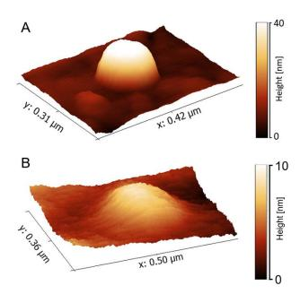
Figure S1. AFM height maps of drug filled liposomes deposited via nES GEMMA (A) and a simpler deposition method consisting of placing a droplet on the substrate before letting it dry in an unforced way at room temperature (B)
